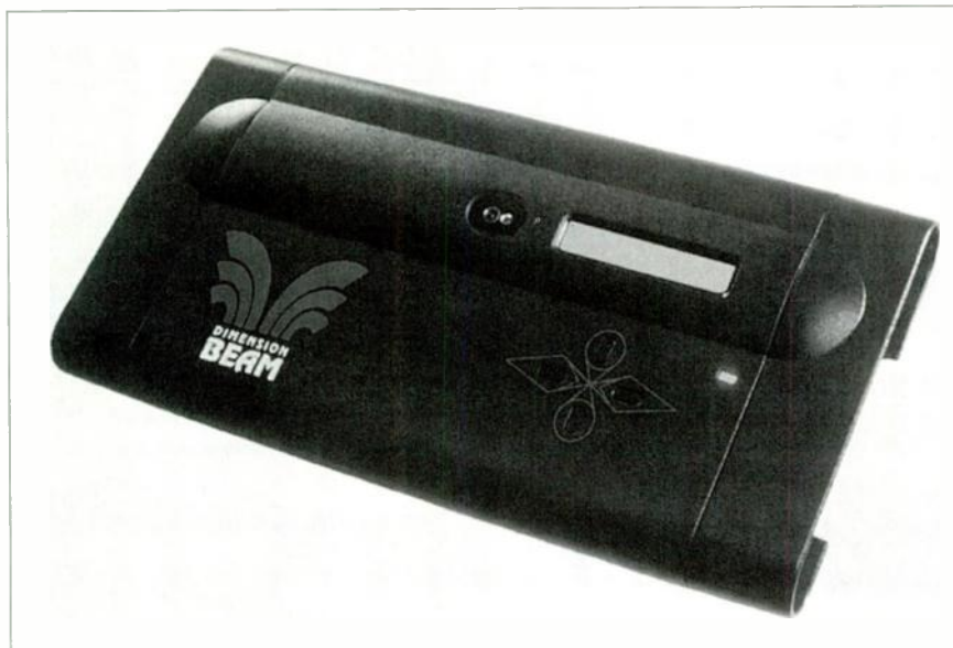
Interactive Light's Dimension Beam uses infrared light to sense movement, which it translates into user-defined MIDI messages. It can be mounted on any mic stand.
