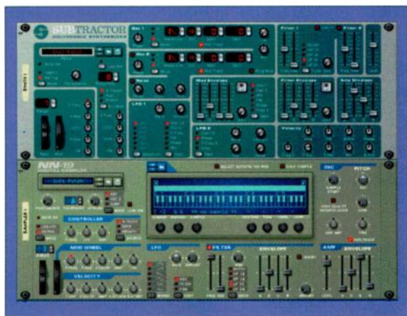
FIG. 3: The Subtractor polyphonic synthesizer and NN-19 sample player are the typical modules of choice for pitched instruments and sound effects. An oscillator phase and a second filter help distinguish Subtractor from most software synths. The sonic architecture of the NN-19 is similar but simpler.
