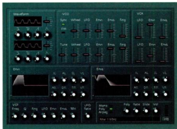
FIG. 2: CesSynth1 is a virtual-analog subtractive synth featuring mixed waveform oscillators, envelopes with adjustable level and rate for each stage, and a 4-pole resonant lowpass filter. Most filter and oscillator parameters can be modulated by the LFO and either envelope.
