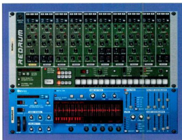
FIG. 4: Most rhythmic material is created using Redrum (top) and Dr. Rex (bottom). Redrum enhances the standard drum-machine model by offering special control effects on different channels. Dr. Rex is a powerful sliced-loop player and offers extensive control over slices and the global loop.
