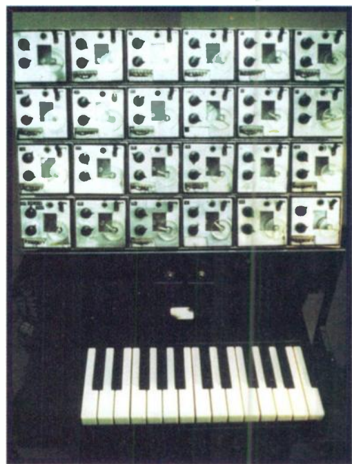
FIG. 8: This later version of the Oscillator Bank (1961) had a touch-sensitive keyboard.
