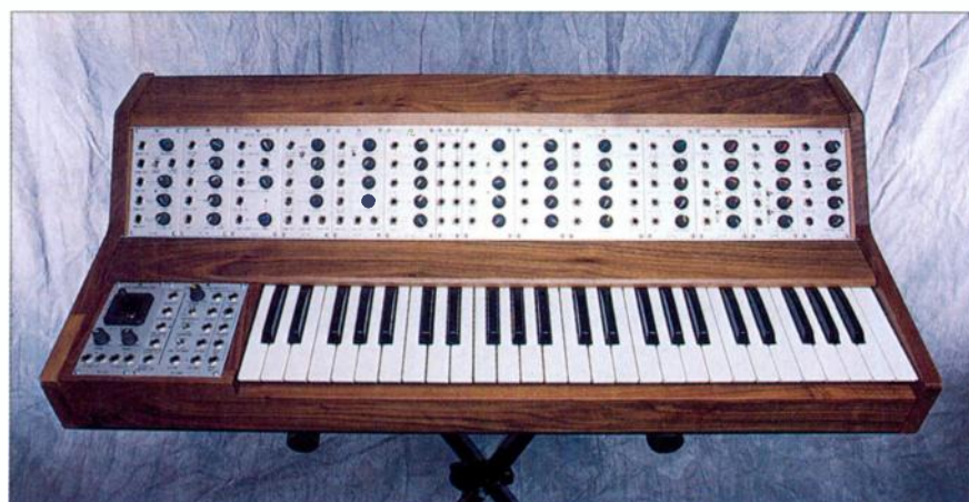
FIG. 1: With its classic good looks, the monophonic Sorcerer provides a foundation for constructing a modular system from a large selection of synth modules.
