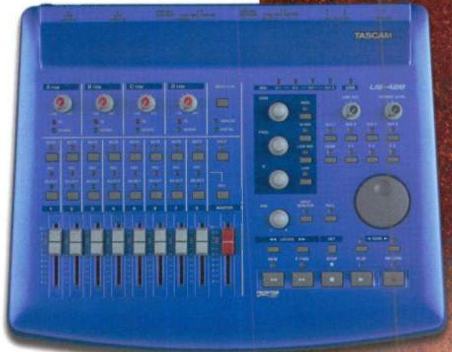
FIG. 1: The Tascam US-428 includes a full complement of faders, buttons, and knobs designed to give you tactile control over your music-software mix functions.
