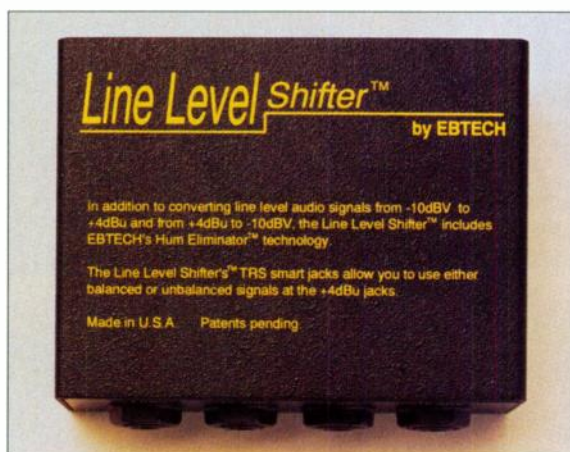
FIG. 5: The Ebtech Line Level Shifter changes the signal levels of eight outputs from -10 dBV to +4 dBu and vice versa. It also automatically converts from balanced to unbalanced (and back again), depending on whether you use a TRS or TS plug.
