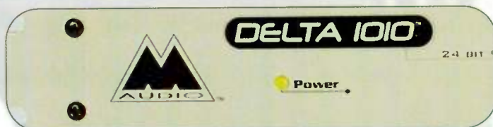
DELTA 1010 - 10 in/ 10 out PCI digital recording system.
