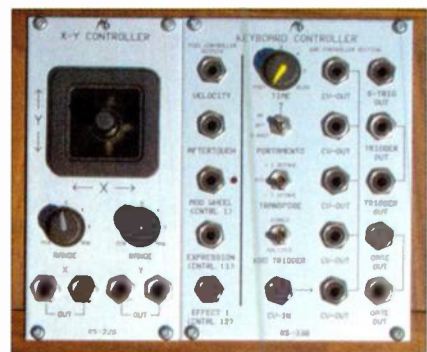
FIG. 3: The RS220 (left) features a joystick with separate CV outputs for the x- and y-axes. The RS330 module (right) routes control signals from the keyboard to the other modules.
