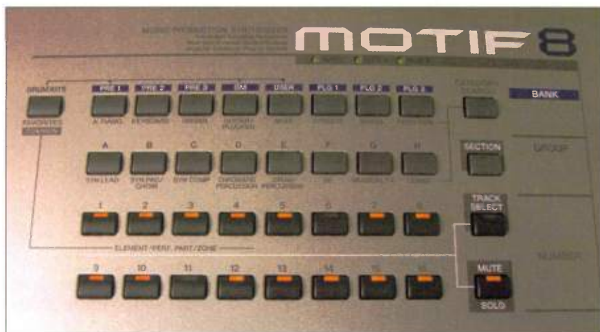
FIG. 2: This 32-button grid is the key to piloting the Motif. Here the Motif is in Track-Mute mode; other modes let you quickly select sounds, tracks, sequences, and oscillators.
