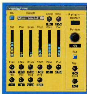
FIG. A: The Kaleidophone4 Ensemble in Reaktor is a granular resynthesizer that randomizes all grain parameters. It uses a collection of audio files (called a map ) for its sound source.
