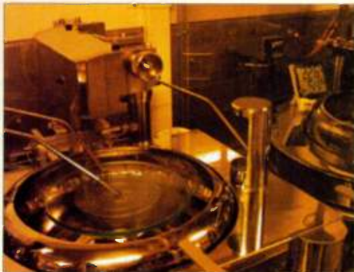
FIG. A: Among the many steps in the creation of a CD is the process of washing the coated master disc. Following this step, a thin layer of silver will be applied to the disc in order to make it electrically conductive.
