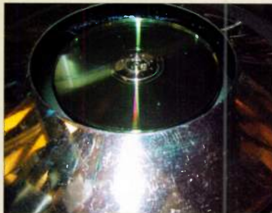
FIG. B: Dye coating a CD is done using a process called spin coating . The disc is spun at a very high speed so the coating is applied evenly.
