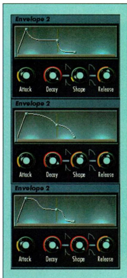
FIG. 2: Attack 's envelopes feature a continuously variable range of shapes for the decay and release segments, ranging from concave (top) to convex (middle) to S-shaped (bottom).
