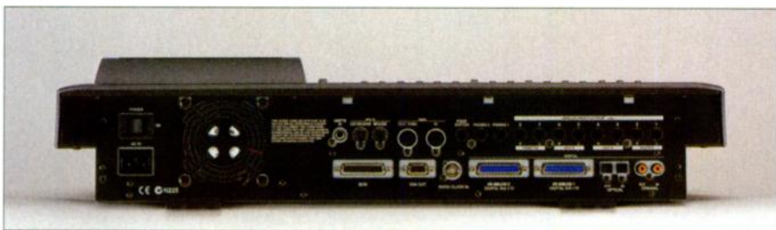
FIG. 2: To the right of the VS-2480's power switch, AC connector, and fan exhaust vent are jacks for SMPTE input, a mouse and a computer keyboard, MIDI In and Out/Thru, a footswitch, two pairs of stereo headphones, and four pairs of balanced analog audio outputs. Below those are ports for SCSI I/O, VGA out, word-clock in, R-Bus I/O, and optical and coaxial S/PDIF I/O.
