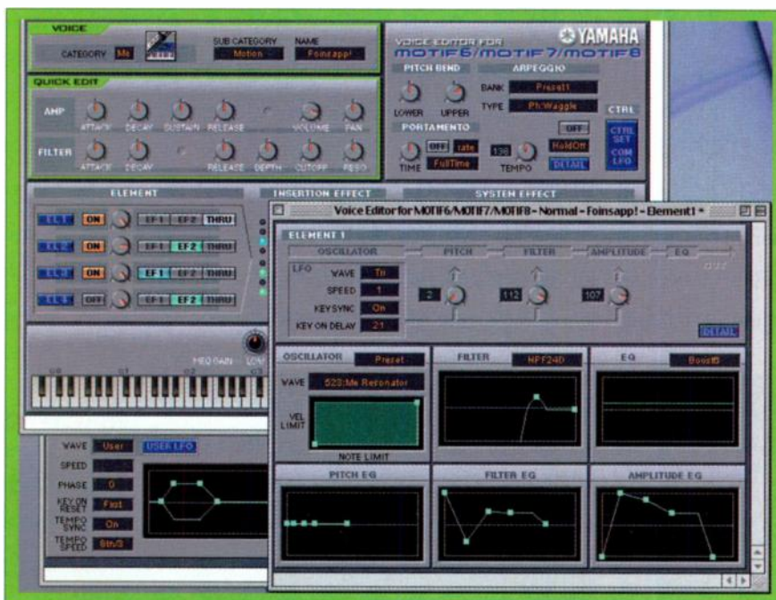
FIG. 4: A basic Motif patch, called a Voice, has as many as four oscillator-filter-amplifier layers called Elements. This shot from the bundled Voice Editor shows the envelope settings for a single Element.
