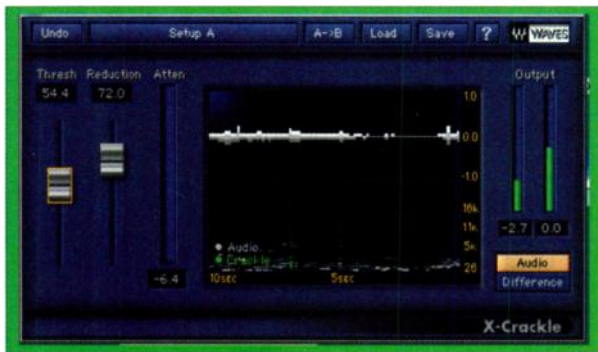
FIG. 2: Crackles detected in X-Crackle are shown in green below the audio waveform. The user can toggle between monitoring the audio output and monitoring the amount of crackle removed by pushing the Difference button.
