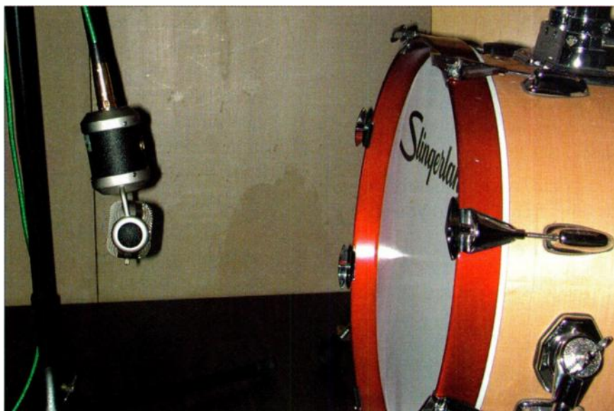
FIG. 1: For a natural sound when miking a double-headed jazz kick, position the mic back a bit from the drum to allow space for the low frequencies to develop. The mic will pick up considerable bleed from the kit, so a high-quality, large-diaphragm condenser is the mic of choice. Here a Blue Mouse captures the punchy tones of an 18-inch bopper.
