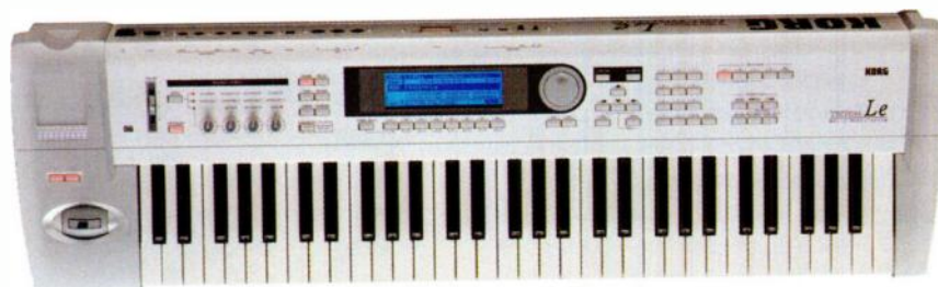
With the optional sampling board, Korg's Triton Le keyboard workstation can load WAV files from CD, process them through the synth engine, and assign sections of the new samples to keys.
