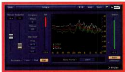
FIG. 4: In this example, a profile (white line) of the residual noise of a vocal track has been created with the Learn button. Judicious control of the Threshold and Reduction sliders in X-Noise completely removed the noise on the output, shown by the green line.
