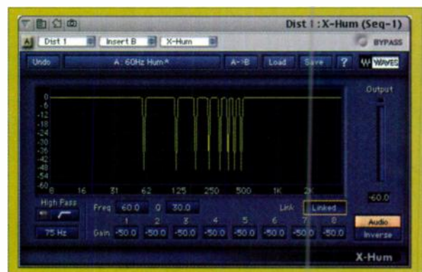
FIG. 3: X-Hum is perfect for removing static noises, such as hums and buzzes. Here the 60 Hz Hum-Removal preset is cleaning up a guitar track from a rig with grounding problems. The steep notches are harmonically related to 60 Hz, which removes the overtones of the hum, as well. The frequencies can be linked, as above, or set independently.
