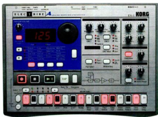
FIG. 4: The bitimbral, duophonic Korg Electribe A blends analog synthesis with pattern-based sequencing.
