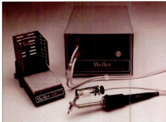
FIG. 2: This Weller DS 800 electronic desoldering station provides a closed-loop, temperature-controlled hollow tip through which solder is sucked into a reservoir by an internal pump.
