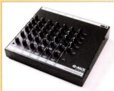
FIG. A: The Oz Audio Q-Mix HM6 is a handy headphone matrix mixer that can drive six pairs of headphones. A simple, affordable, and rugged solution for setting up a More Me mix, the HM6 provides stereo main inputs (for the baseline mix), four separate "inject" inputs, and a separate effects send with stereo returns.
