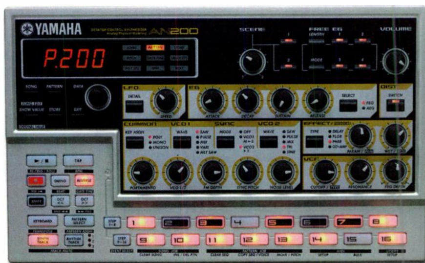
FIG. 11: A member of Yamaha's Loopfactory family, the AN200 is an analog-modeling synthesizer that features sampled rhythm instruments and phrase-based sequencing.
