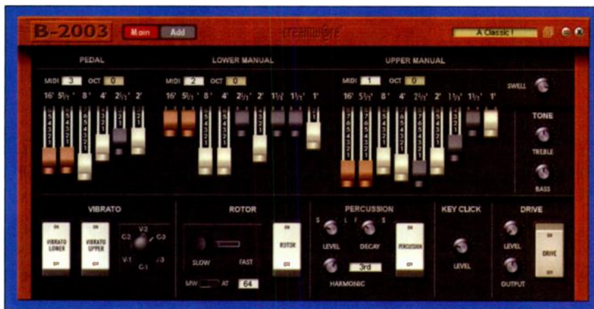
FIG. 5: The drawbars on Noah's Hammond organ model exist only in software, but you can control them from a MIDI slider box.
