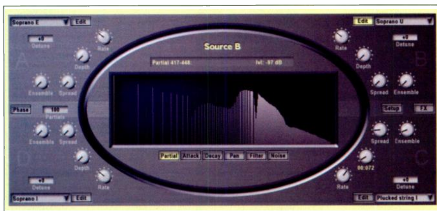
FIG. 2: Cube allows you to control the amplitudes of as many as 512 partials. Each of its four Sound Sources has its own parameters for the partials and for the major sound-processing functions.
