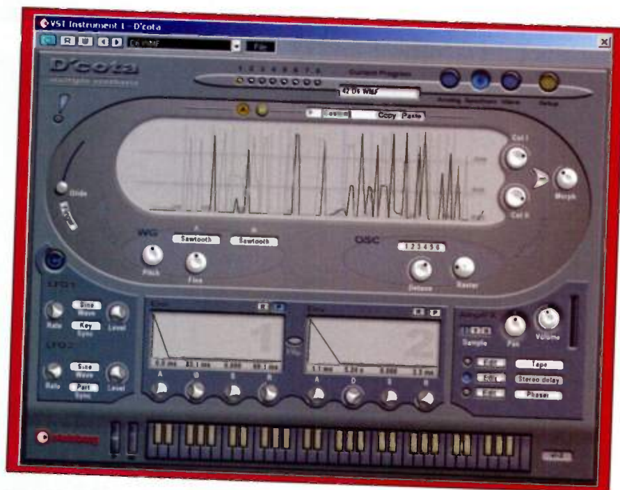
FIG. 1: D'cota's three synth panels (including the Spectrum display, shown here) appear in the upper half of the window. The envelopes, LFOs, and effects in the lower area are common to all three panels.
