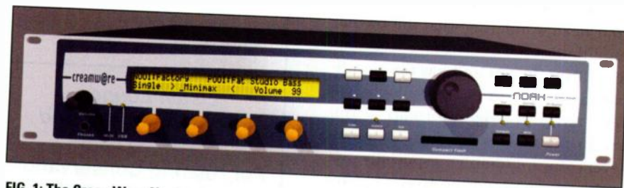
FIG. 1: The CreamWare Noah brings virtual synthesis capabilities out of your computer and into your equipment rack. Its sound engine depends entirely on the software you load into it.
