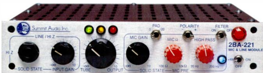
Summit Audio's 2BA-221 is a preamp with mic-, line-, and guitar-level inputs; a knob to vary the mic input's impedance; and simultaneous solid-state and tube outputs. For maximum boost, mic preamp gain is 58 dB and tube output gain is 35 dB.
