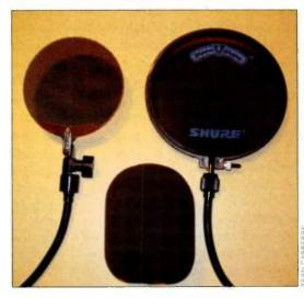
FIG. 4: To reduce plosives, you can use a metal pop filter (left), a foam windscreen (or "sock," center), or a mesh pop filter (right). Pop filters are better in most situations because they don't attenuate highs as much as foam screens do.
