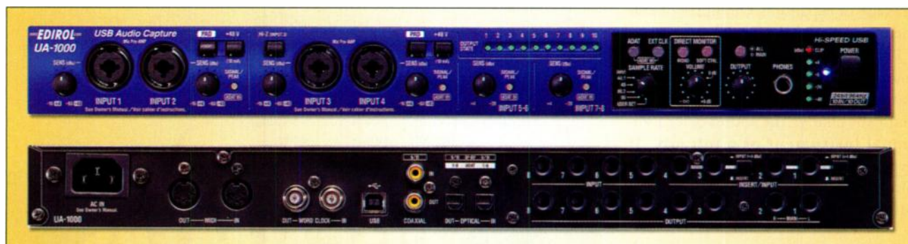
FIG. 1: The Edirol UA-1000's front panel features four combination XLR/TRS inputs with preamps and phantom power. The back panel handles the rest of the connections, with analog audio, digital audio, word-clock, and MIDI I/O.
