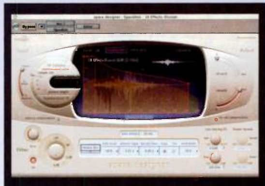
FIG. A: Emagic's Space Designer reverb plug-in combines real-time convolution with filter and envelope controls. Its sound ranges from highly realistic to bizarre and unusual.
