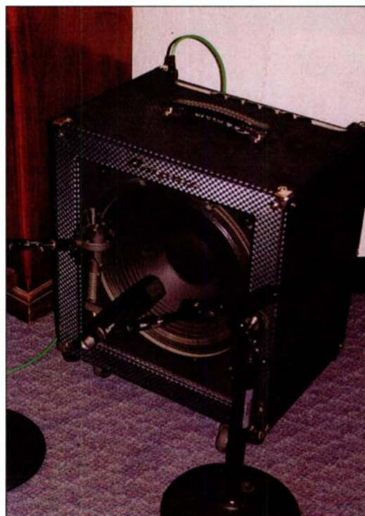
FIG. 4: One of Wakeman's preferred cabinet-miking configurations consists of a Sennheiser MD421 aimed at the center of the speaker, and a Royer R-121 ribbon mic a short distance back and off to the side.
