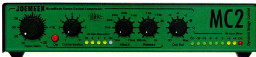
FIG. 3: Don't be fooled by the diminutive size of the Joemeer MC2 stereo compressor. This elfin box has gigantic powers. Featuring photo-optical control and an auto-variable slope (ratio), the versatile MC2 is perhaps the best-sounding inexpensive hardware-based compressor available—that is, if it's attitude you're after. It works especially well on drum subgroups and room mics.
