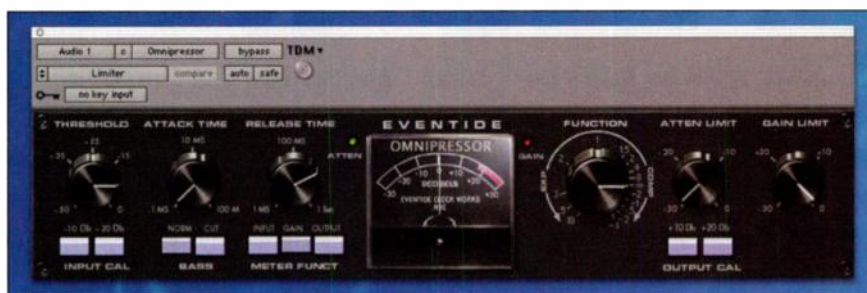
FIG. 3: The Omnipressor compressor's Function knob allows for a wide variety of compression types, including dynamics reversal.
