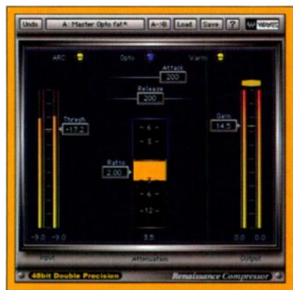
FIG. 1: The Waves Renaissance Compressor is a cross-platform plug-in that can emulate both VCA-based and optical compressors.
