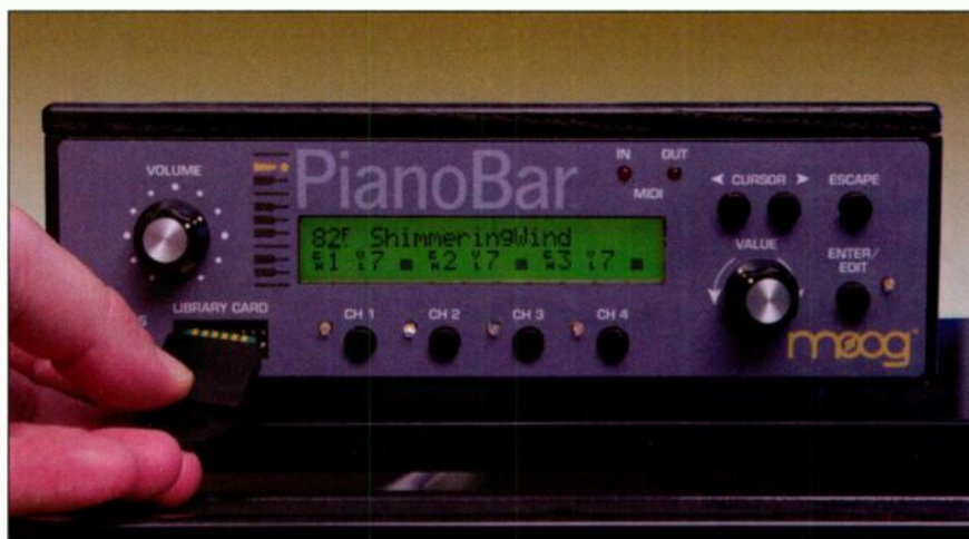
FIG. 2: The Control Module, a GM2-compatible sound source, stores 100 multitimbral Setups in addition to converting sensor signals to MIDI data.
