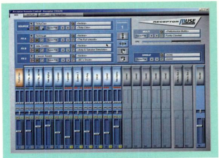
FIG. 5: Muse Control software provides a graphic user interface for programming Receptor's mixer as well as individual plug-ins that use their own graphic user interfaces.
