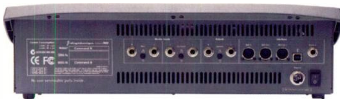
FIG. 2: The Command|8 rear panel includes audio and MIDI I/O jacks as well as USB and footswitch input jacks.
