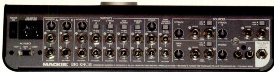
FIG. 2: The rear panel features multiple I/O as well as switches and knobs for adjusting various inputs and outputs from -10 dB to +4 dBu.
