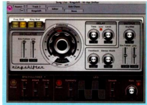
FIG. 4: The new Ringshifter plug-in offers ring modulation and frequency shifting.
