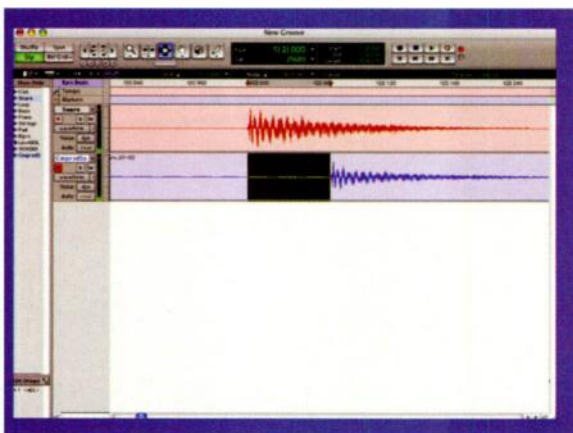
FIG. 2: Recording a processed signal allows you to see the amount by which the unprocessed signal can be offset in order to align the newly processed signal with other tracks.
