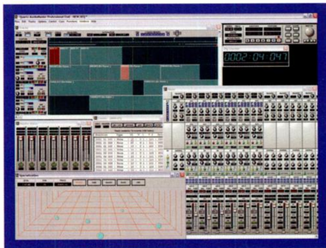
FIG. 6: Quartz AudioMaster's interface should be familiar to anyone who has used a sequencer before. Its feature set includes plenty of audio and MIDI tracks along with an interesting Specialization window.
