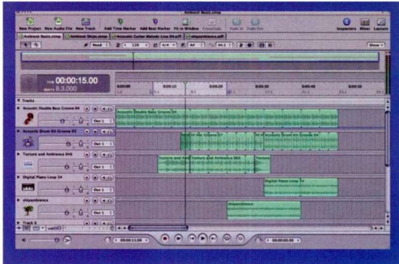
FIG. 1: Soundtrack Pro's Multitrack and Waveform editors share the same Project window. Individual projects are accessed using the tabs along the top.
