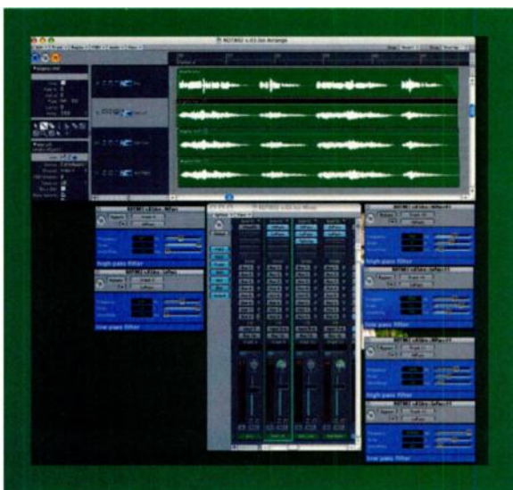
FIG. 1: With the use of high- and lowpass filters, the frequencies of the wet file can be split across several tracks. Here, they are also panned and offset. The center track is being processed with a tape-delay plug-in.
