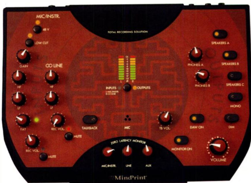
FIG. 1: The MindPrint TRIO combines input and monitoring functions that might otherwise be missing from a mixerless personal studio.
