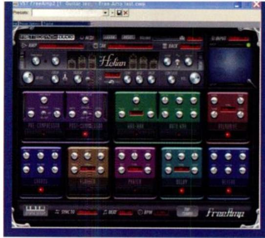
FIG. 4: Fretted Synth Audio's FreeAmp 2 is a fully featured freeware amp-, cabinet-, and effects-modeling VST plug-in for Windows.
