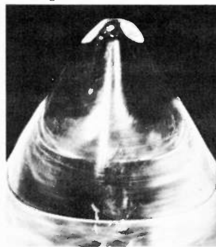
No sign of wear after repeated plays with a stylus at a downward tracking force of 1.5 grams. The microscopic dry lubricant coating (Sound Guard) reduces the friction between stylus and groove modulations, without filling in minute groove variations.
