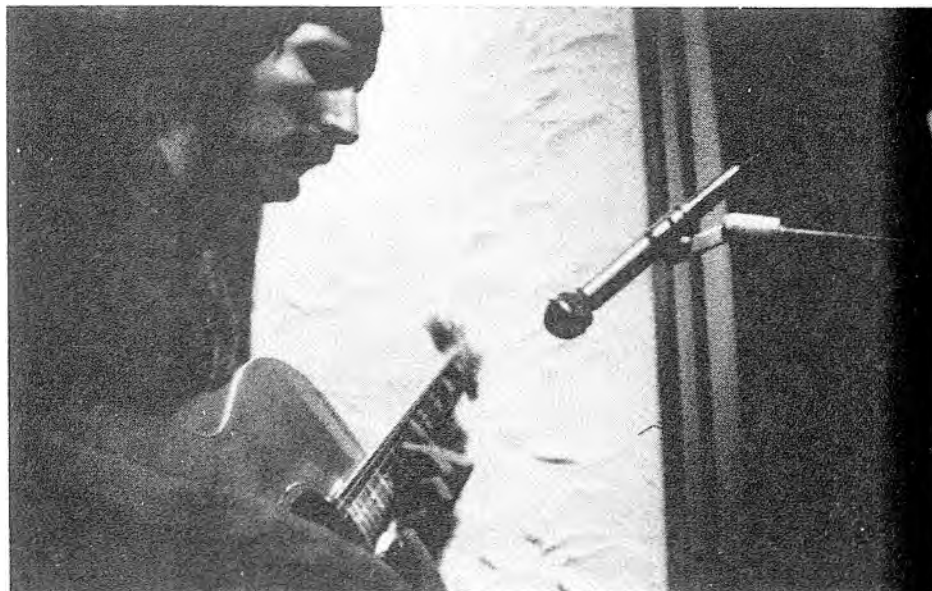
Pic. 2: Microphone position for steel string guitar.
