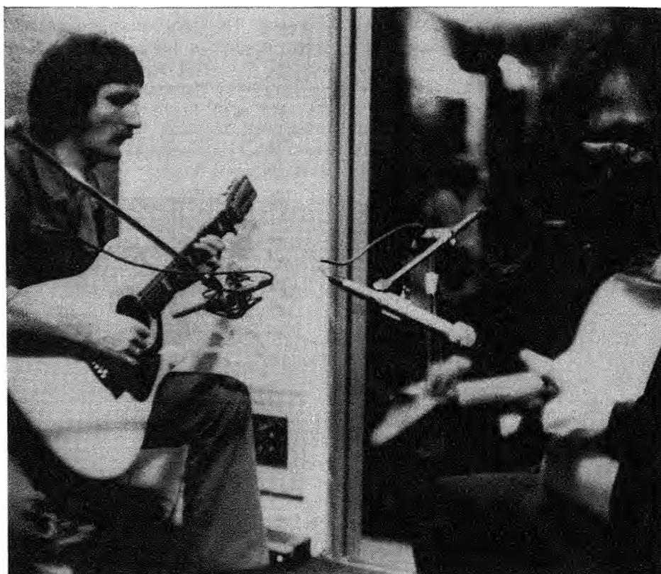
Pic. 5: Microphone position for guitar duets.
