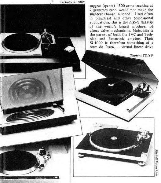
whose air of professional simplicity fails to hide its obvious engineering superiority. Lavish execution of the EPA100 tone arm includes nitrogen hardening of a dual-layer titanium arm tube, a 20-ruby gimbal suspension at the pivots, variable and independent damping in vertical and lateral planes.
