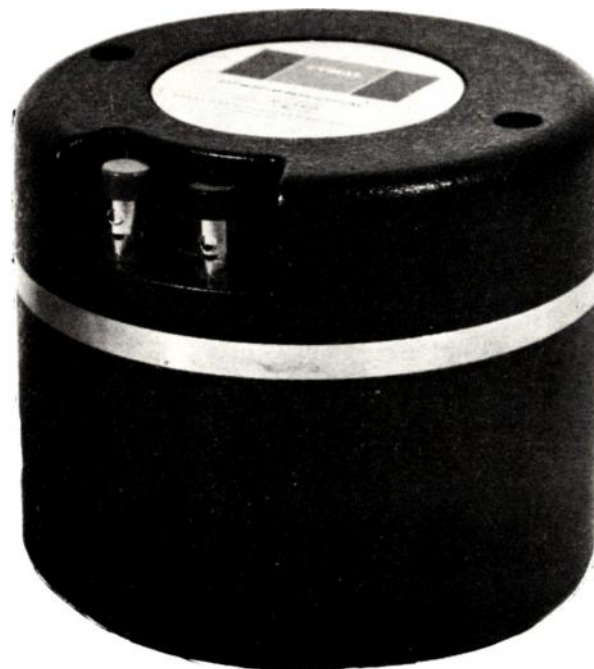
M100 50 watts RMS Frequency response 500–1800 Throat Diameter 1" 16 \Omega
