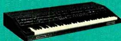
Sequential Circuits' Prophet T8 is a completely touch-sensitive (velocity and pressure), fully programmable eight-voice polyphonic synthesizer. Its 76-note wooden keyboard (A to C) has been packaged in a compact design weighing less than 60 pounds, and all together the T8 sports 128 programs. A built-in real-time sequencer has been included; with a memory capacity of over 600 notes, it will record up to eight separate sequences.
