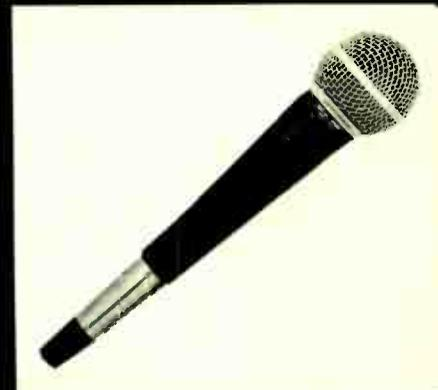
Shure's ubiquitous SM58 has an impedance of 150, a frequency range of 50Hz to 15kHz, weighs 10 $\frac{1}{2}$  pounds and comes in a gray enamel finish. Other features: -75dB sensitivity at 1kHz open circuit, and cable connector type is bare. But what so many vocalists seem to value most is the SM58's ruggedness.
