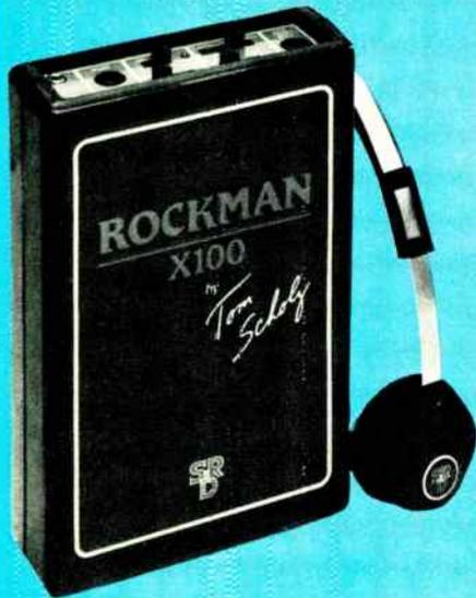
*On-Go for Your Life*. West utilized the Rockman, Tom Scholz's original. The newer model is the X100, which features four equalization settings; high-energy distortion setting, providing plenty of overdrive and sustain; edge setting; gain control; two "clean" settings; solid-state reverb; stereo echo; and the highly acclaimed Scholz stereo chorus.
