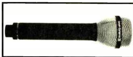
The **Beyer M 69** is a professional dynamic moving-coil microphone with wide response and high output. It has a hypercardioid polar pattern, smooth 50Hz-to-16kHz frequency response, brass case, and comes with a pop screen and a swivel adaptor. Retail price is \$165.
