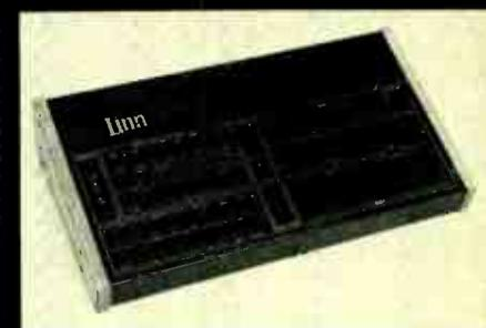
Striking fear in the hearts of drummers the world over, Roger Linn's revolutionary invention features 98 rhythm patterns, user-changeable drum sounds, 16 separate drum outputs, a 16-input stereo mixer, tunable drums, external triggers and adjustable error correction. Easy to use, it was designed for nontechnical musicians.
