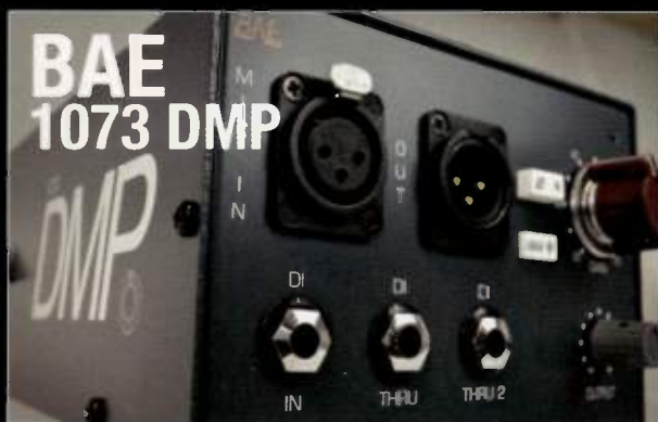
Desktop version of the 1073MP mic pre with DI input, two DI through outputs and polarity switch
