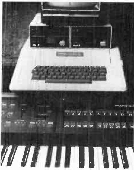
Left, some of Fender's newest microphones. Above, the Fender Chroma synthesizer, complete with an interfacing Apple II computer system and video screen.
