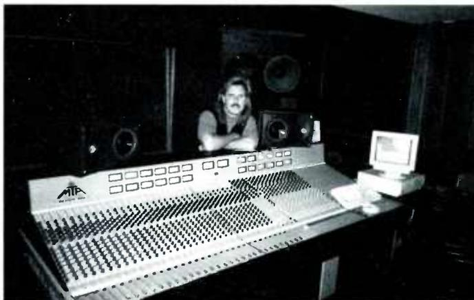
**Producer/studio owner Dino Maddalone is pictured with the new MTA Series 980 recording console. Designed by Malcolm Toft in London, this console is a fully computer automated recording/mixing desk, with Uptown moving faders, and was specifically designed and built for Maddalone's Dino M III Recording Facility in Torrance.**
