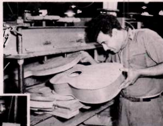
2. Glueing tops and backs to the sides.
