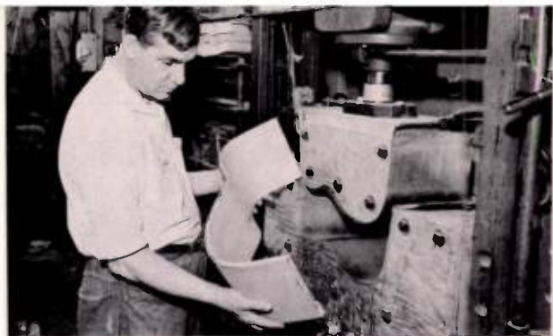
1. Moulding of the guitar sides, done under extreme heat and pressure on specially constructed forms
