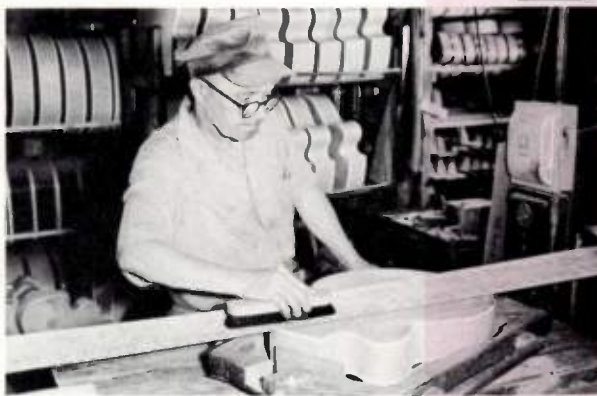
3. Fine sanding of the bodies done by conveyor belt sanders.
