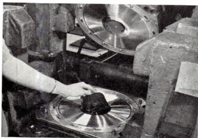
7. Twist of wrist brings stampers together. Hydraulic pressure, combined with heat supplied by live steam passing through press, quickly mold the biscuit into a record. Cold water circulates through the block, cooling and hardening record simultaneously.
