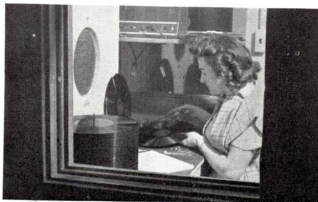
10. Girl plays record for first time. Test booth operator checks record for quality and freedom from extraneous noises, and such imperfections as scratches or ticks. If record fails in any part of examination, entire stamping will be tested.
