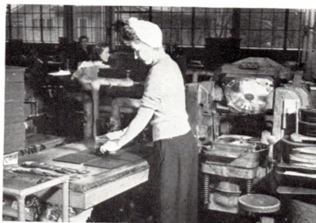
9. Excess material is peeled off edges. The pressure of the stampers has caused excess material to push over the edges of the record. Here the girl operator trims off this excess. The edges of records have become important with the advent of record changers.
