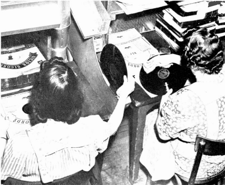
As records come down from edging machine they are put into envelopes, and, having passed test, are sent to shipping department
