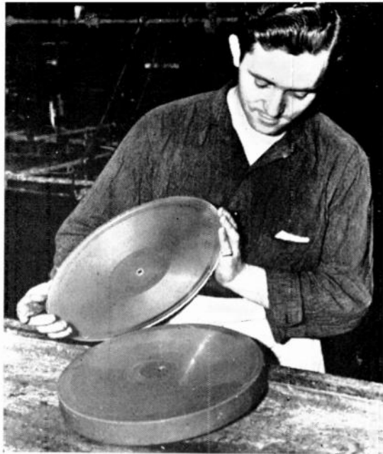
The copper plate, called "master," is pried off the wax disc. Later on it will be nickel plated and a test record will be pressed from it
