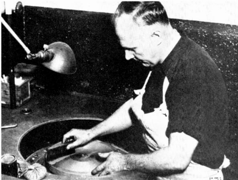
The disc in front of the gold sputtering chamber (other pages) is being groomed for the future master print. Next, in the process of transformation from wax to record the disc is coated with an even layer of bronze powder, later to be replaced by silver
