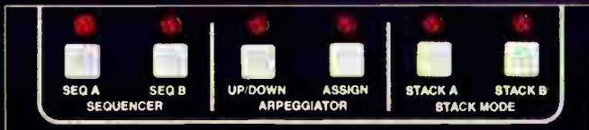
Or you can call upon one of the Six-Trak's totally new features like "Stack Mode" which lets you layer up to six different instrument sounds on top of each other so that your solos feature unique, new "Super Patch™" sounds.
