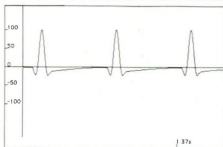
Sustaining portion of digital Phase Distortion trumpet patch: Note the very long "dead" areas between wave cycles, similar to that found in the beginning of the real trumpet sound.
