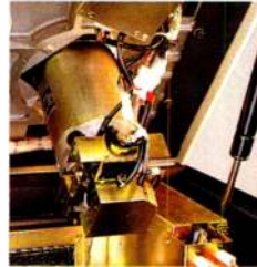
Reel motors that approach one horsepower are driven by pulse width modulation amplifiers to tape speeds up to 174 ips.
