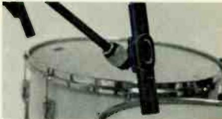
M 201 combine carefully regulated proximity effects with precisely controlled polar patterns. By varying placement and distance, you can capture each drum's character and personalize the player's sound.
