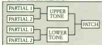
**LA Synthesis Explained/**LA Synthesis is component synthesis on the highest order. To create complex sounds, the D-50 starts with a very simple premise—build sounds from the ground up by combining different types of sounds
