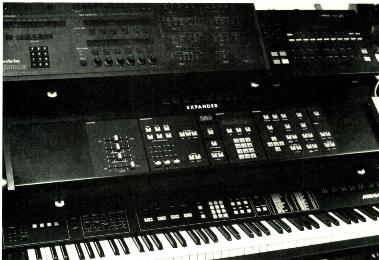
This new Berklee College electronic music work station mixes all three types of MIDI-accessible sounds: analog (an Oberheim Xpander), sampling (Kurzweil 250) and digital (a Yamaha TX816 rack off-camera), plus digital drums (RX11).
