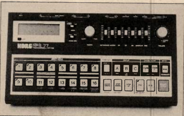
Korg's KPR-77 Programmable Rhythmer stores up to 48 two-measure patterns and six 256-measure chains which can be combined to create three 512-measure chains. Voices may be programmed in real-time or beat by beat, with a seven-channel mixer and independently-controlled accents for control of dynamics. Suggested list price: $695.00.
