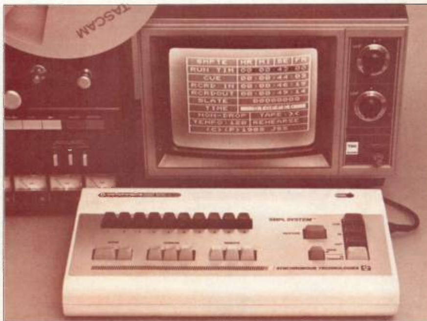
Synchronous Technologies' SMPL System: Computerizing the standard analog tape recorder
