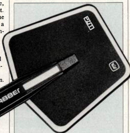
Crown's Sound Grabber PZM™, with plastic casing and boundary plate, is a quality alternative to more expensive metal mics of its kind (approx. $100)
