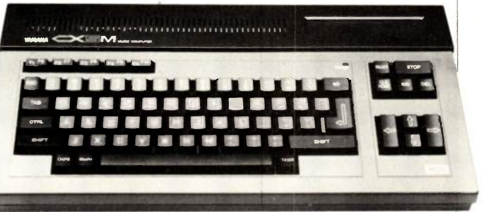
Yamaha's CX5M computer is designed specifically for musical applications (under $500)
