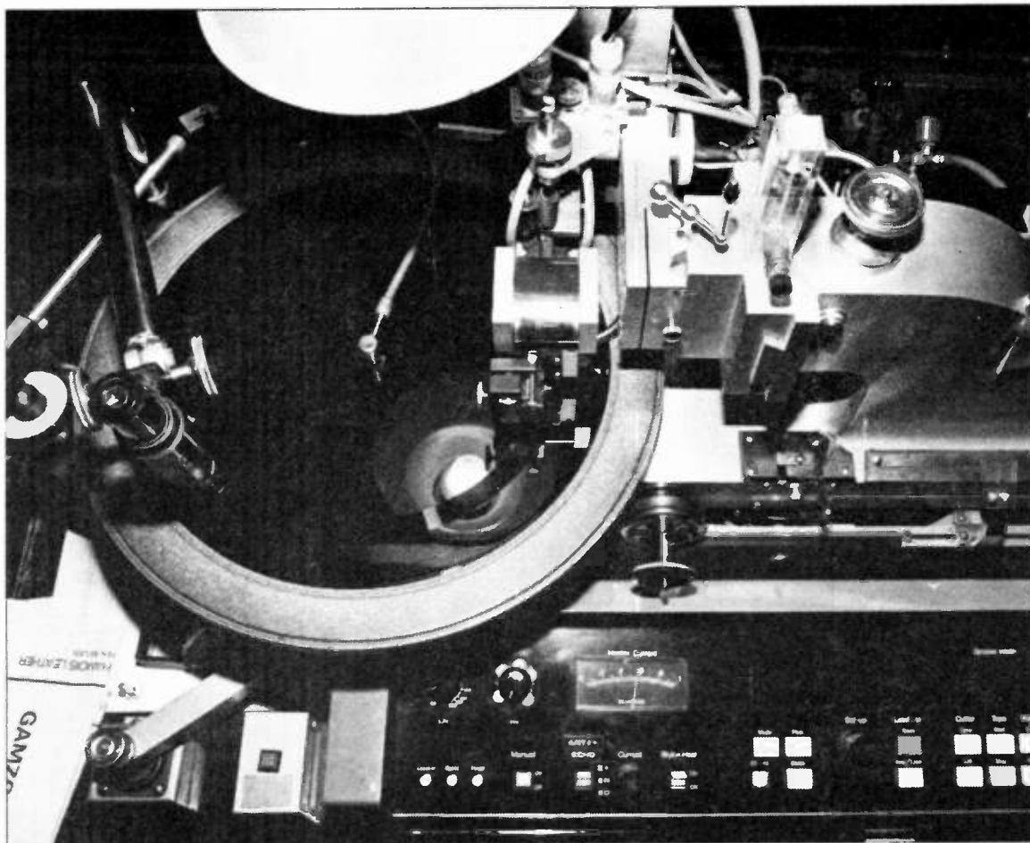
Cutting the master lacquer: the most critical step in the signal chain
