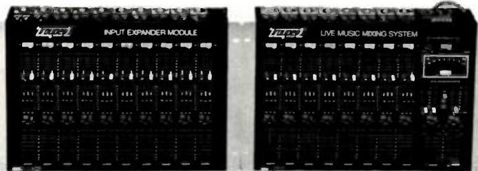
The Trouper I has become an industry standard in the short time since its inception. Serviceable, expandable, easy to operate yet sophisticated, the Trouper I has several outstanding features that set it apart from other mixers, such as a solo system, multiple inputs and in/out jacks on each channel. Write for details or ask your dealer.
