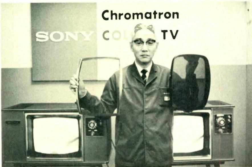
COLOR SELECTING GRID used in Sony's 19-inch "Chromatron" color set (left), is compared with shadow-mask by company's Akio Morita. Set will be sold in Japan next spring, but company does not plan to export "for a while."
