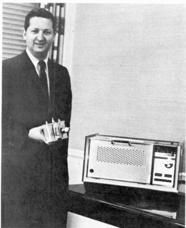
TABLE MODEL ELECTRONIC OVEN developed by Amperex Corp. is shown here with Ed King, product manager. King holds ceramic and metal magnetron which is heart of company's electronic oven system. Product manager thinks table oven, designed by Banka Mango, can be sold for \$400.
