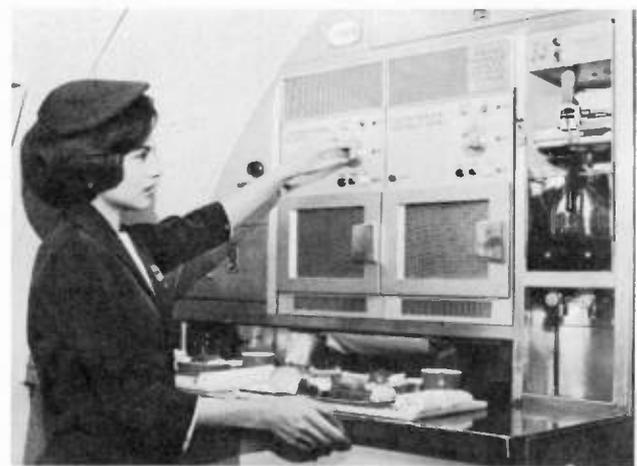
*JET ELECTRONIC OVEN — Special oven configuration developed by Litton Industries in co-operation with Trans World Airlines, Inc. is shown here. Installation of unit in TWA's entire jet fleet is scheduled by fall. Ovens are expected to not only reduce cooking time and improve food quality but also to permit airline to offer wider menu selection and more personalized passenger service.*
