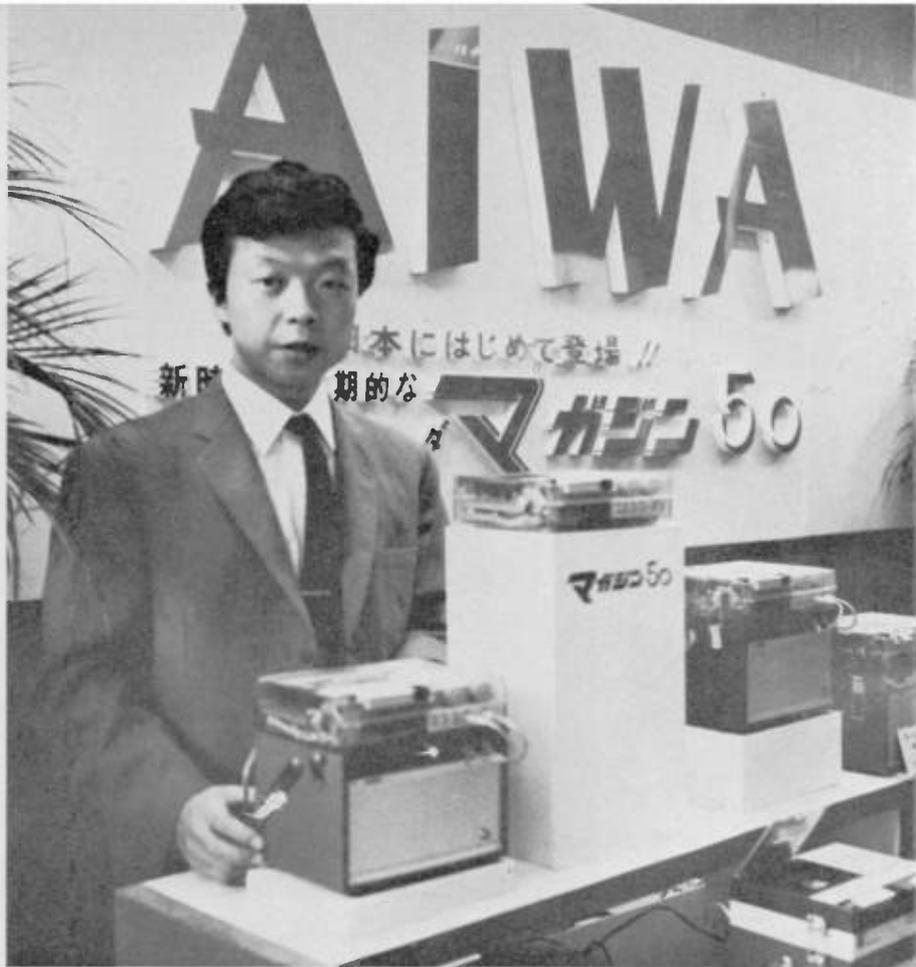
MAGAZINE TAPE RECORDER, with speaker and radio in base is shown by Aiwa Co. Ltd. Reversible cartridge plays for 15 minutes. Unit sells for about \$62.50 in Japanese market.
