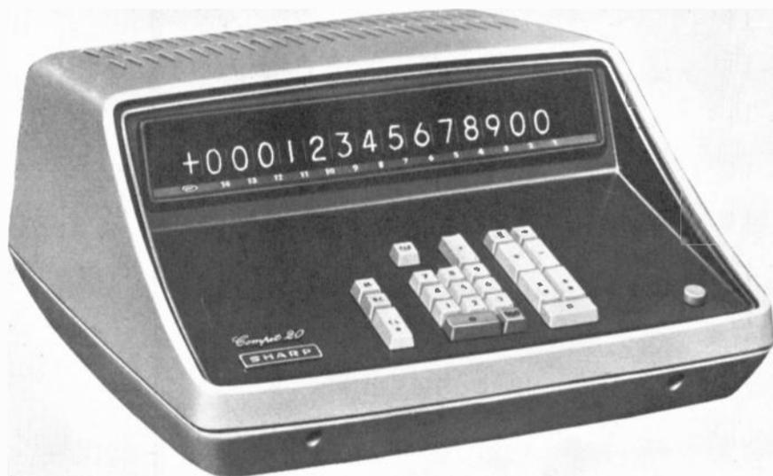
**ELECTRONIC DESK Calculator, "Compet 20,"** said to perform any calculation within 14 digits in a moment. Equipped with 10 keys in all, unit has guide key to insure blind operation. It also has three-zero key that disposes of three zeros at a time. In all calculations, decimal point is automatically indicated in display board. Model CS-20A is said to retail for little over \$1,000 in Japan. Sharp Electronics Corp., 178 Commerce Rd., Carlstadt, N. J.
