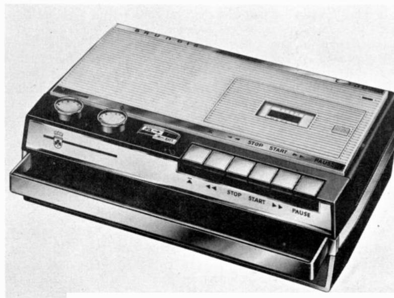
COMPACT MONO tape recorder Model C 100 is scheduled for early U.S. introduction by Grundig. Two-track unit is battery or cord operated.
