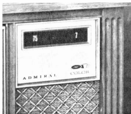
CLOSED: When the panel is shut, all controls are hidden and only the lighted channel indicators, both UHF and VHF, are on view in the front of the set.
