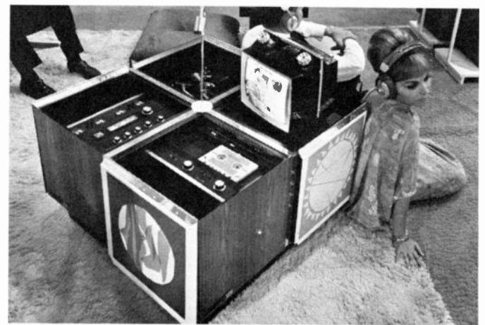
RCA's show-stopper: a modular unit offering transistor tv, radio, stereo tape, and phonograph in a jazzy-looking building-block ensemble. Speakers are extra.
