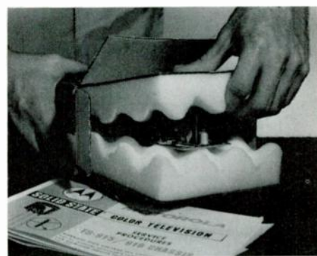
Module is opened by the serviceman in the home; package includes instructions
