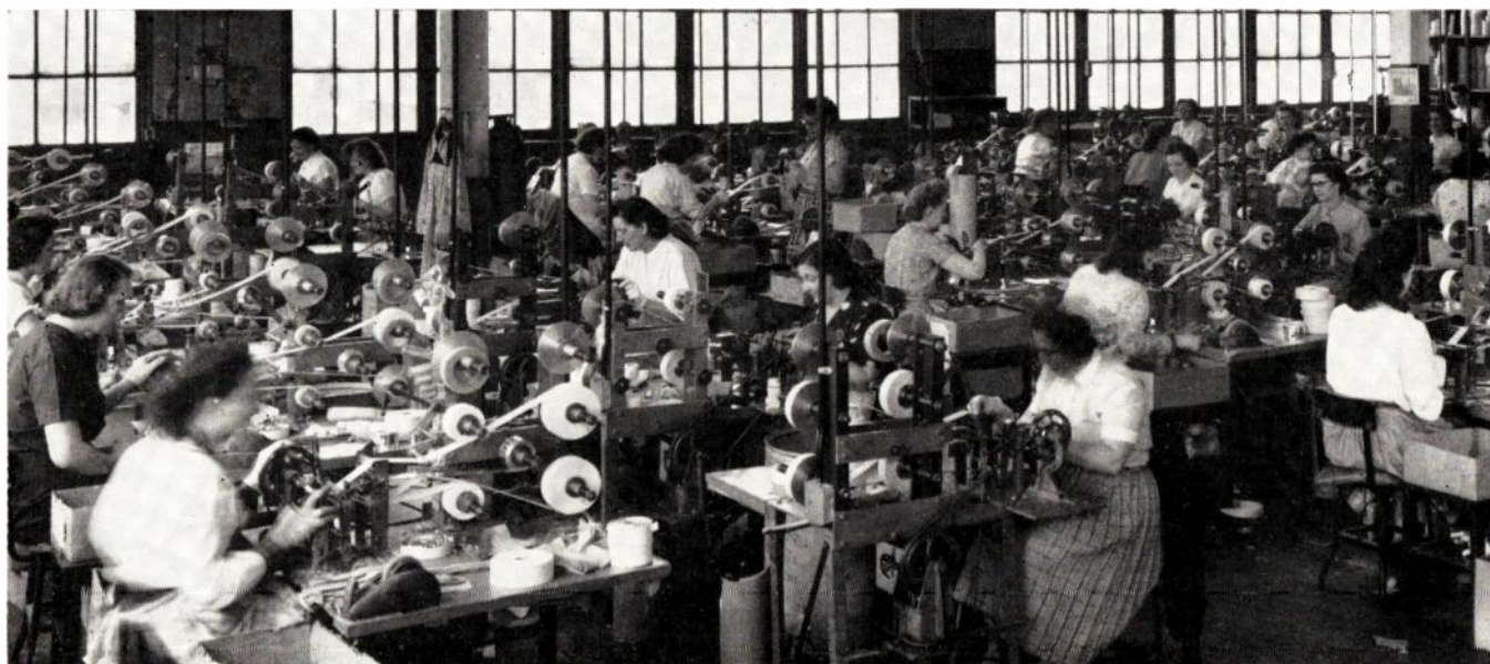
In Pyramid dry electrolytic section-winding departments each machine turns out thousands of sections every day.
