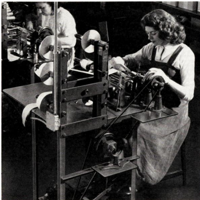
Rubber gloves are worn by operators winding capacitor sections — to prevent foil contamination by perspiration.
