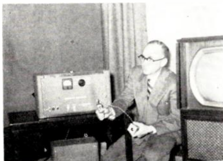
FIG. 4. The two tube decoder unit and key assembly.
