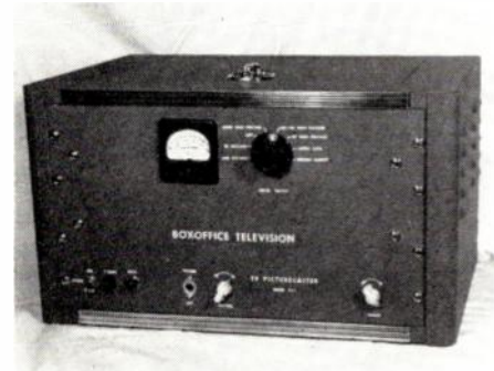
FIG. 1. TV Picturecaster for broadcasting coded and uncoded pictures and sound on VHF channels.
