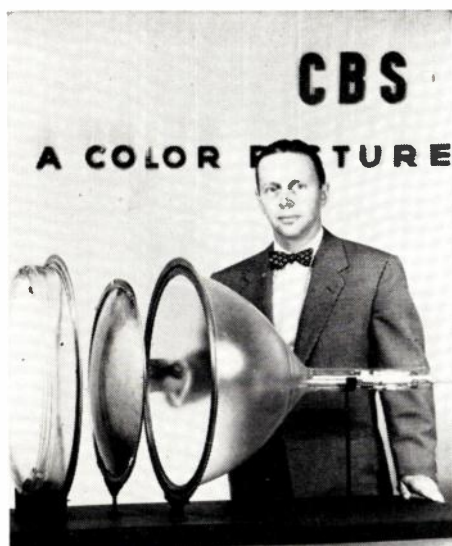
C. F. STROMEYER, President of CBS-Hytron with "205" cross-section. Left to right, parts include: Face plate with tricolor phosphor-dot screen, simple lightweight shadow mask, glass funnel, and electro-magnetically converged three-beam electron gun.
