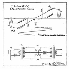
grids are excited, as shown below, a pulse of plate current flows for alternate half cycles, in the plate circuit of each tube. Since these pulses of plate current of each tube do not flow during the same half cycle each current will set up a strong D. C. field necessitating the use of a large core for T<sup>a</sup> in order to minimize the possibility of core saturation.
