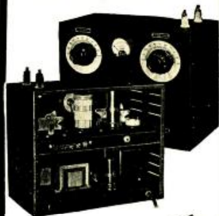
A simple controlled noise generator—hard on programs but good for tests. Aerial connects to buzzer contact.
