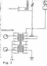
• For best results an oscilloscope should be used for adjusting the grid excitation. The variable resistor should be connected between taps 1 and 2 and adjustments made. If suffi-cient grid modulating voltage is not obtained the position of the resistor may be changed to 2 and 3, 3 and 4, etc.
