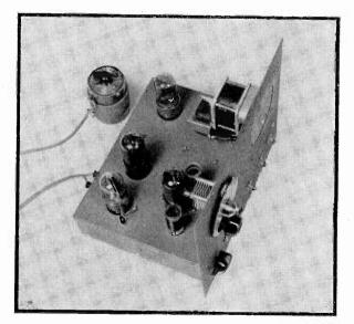
Interior View, Showing Placement of R-F and Oscillator Coils, A-F Tube, and Loud-Speaker.
