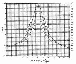
Fig. 1. Universal Resonance Curve, With Corresponding Phase Angles.
