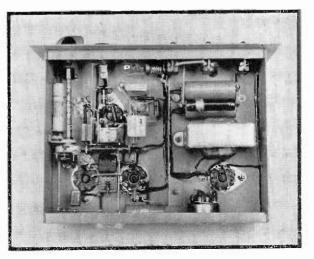
Under-chassis View. Showing Shield Plate Between Power Supply and R-F Components.
