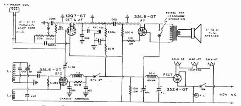
Circuit Diagram of Complete A.C. Frequency-Meter-Monitor.
