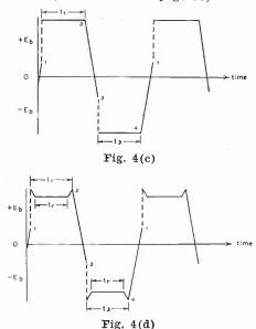
same conditions holding true for the points 4 and 1. This would also hold true, again, for the self-rectifying type of vibrator operating on no-load. "No-load" does not mean the removal of the first filter condenser, however.
