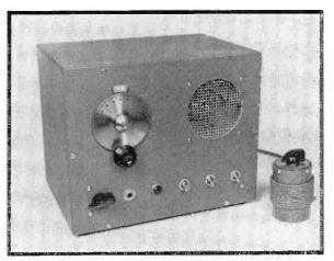
Front View of A. C. Frequency-Meter-Monitor and Pick-Up Coil. The Tuning Condenser Mounted Inside the Coil is Optional and Not Usually Required.
