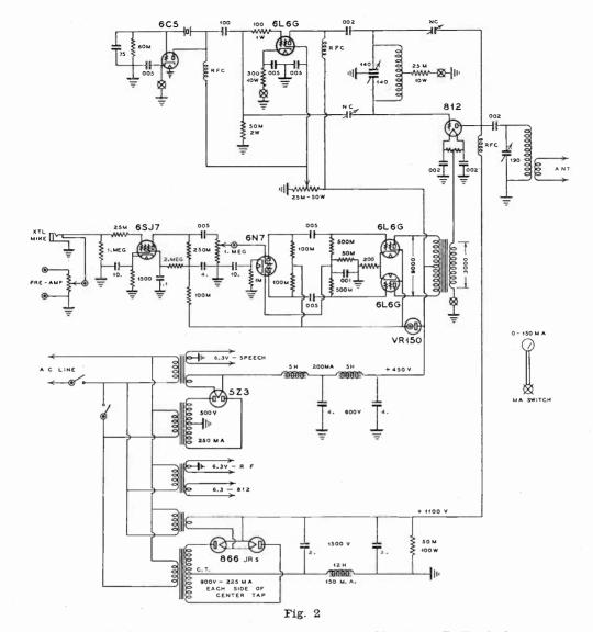
Circuit Diagram of the Grid-Neutralized Cathode-Modulated Radiotelephone Transmitter discussed in this treatise.
