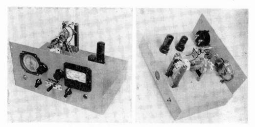
Front and Interior Views, Showing Variable Antenna Coupler Details.
