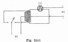
There are two ways of applying energy to a drive coil. A separate set of contacts can be installed on the reed as shown in Fig. 2(c), in which case the operation of the driving circuit is exactly the same as the circuit of a common household buzzer or bell. Fig. 2(d) shows the circuit used in Vibrapacks. This is called a shunt driver circuit and eliminates the complexity of the extra contact points, since one set of the regular interrupter points now performs double duty.
