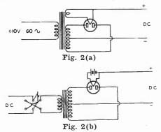
simple method of doing this would be to connect a double pole, double throw switch as a pole reversing switch, as shown in Fig. 2(b). Flipping the switch back and forth will produce an alternating current.
