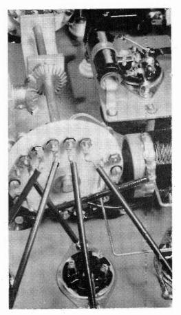
Typical example of engineering design for a band-switching unit in a commercial transmitter. From a photograph of Tecrad's marine application.
