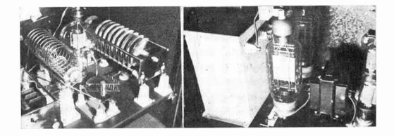
Here is the Kalifornia Kilowatt at W6NZ in all its grandeur. It's an Eimac 450TL, operating us cold as a cucumber with 999.99 watts input. The modulator (right-hand illustration) likewise employs large tubes, but with conservative output, which is one of the reasons why W6SZ's speech quality is tops.
