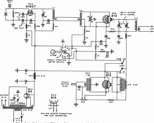
Complete Schematic Wiring Diagram of All-Band, 'Phone-C.W. Transmitter
