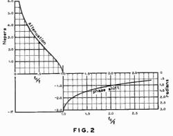
Fig. 2—Characteristic Curves for High-Pass Section.
