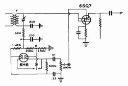
Fig. 1-New Series-Shunt Type Silencer
