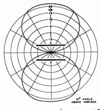
2 DRIVEN HORIZONTAL & ANTENNAS 180° OUT OF PHASE 1A IN HEIGHT ABOVE GND
