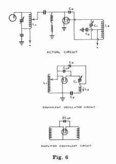
The cure for this form of parasitic circuit is the substitution of a split-stator plate tuning condenser, with its rotor connected to ground. The tendency for a parasitic oscillation is lowered when the grid circuit is tapped across the entire winding of the driver plate coil  $L_1$ .
