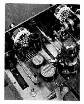
Jones harmonic oscillator with tapped coils and rotary switch for multi-band operation. Two crystals enable the oscillator to deliver output from 160 to 20 meters. A small rotary switch selects either the 160- or 40-meter crystal. Both sides of the crystal are either in or out of service—rather than cutting-in or out the grid connection only.
