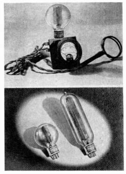
The upper illustration shows an Ohmite Dummy Antenna Resistor, Ammeter and Link Assembly for measuring transmission line losses. The lower illustration shows two Ohmite Dummy Resistors, one for low power measurements, the other for high power (upper illustration referred to as Fig. 9 in text).
