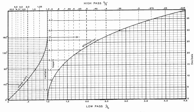
Fig. 1—Chart for Estimating Attenuation and Phase of Frequency Ratios. Also Shows Characteristic Curves for Low-Pass Section.
