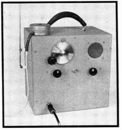
The complete  $2\frac{1}{2}$ -Meter Transceiver in a deluxe carrying case which has ample space for holding the A-, B-, and C-batteries. The microphone is a standard Western Electric F-1 unit, in a special housing.
