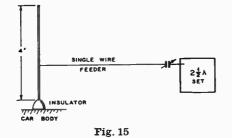
above the base. It is possible to use a single wire feeder with a 4-ft. half-wave vertical antenna in the  $2\frac{1}{2}$ -meter band by connecting the feeder to a point 6- or 8-in. from the center of the rod. The lower end of a half-
