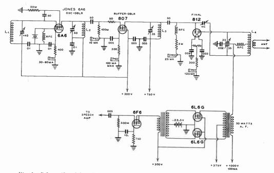
Fig. 1—Schematic wiring diagram, with circuit constants, for r-f portion of 100-watt transmitter—also a suitable low-cost modulator stage.
