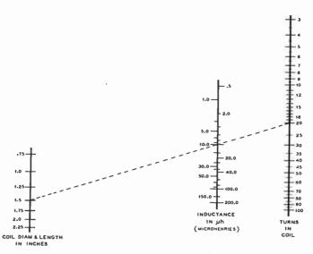
Fig. 2. Coil Calculating Chart.
