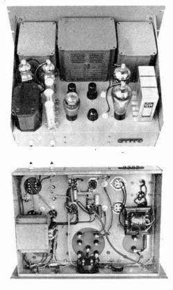
The modulator and speech amplifier, complete from microphone input to modulation transformer, and also including the power supply. UTC components used on this deck.
