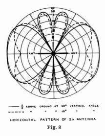
tion, in any direction. The presence of minimums, or *nulls*, in the radiation patterns will help to explain why stations in certain directions can not be easily contacted with a certain antenna installation.
