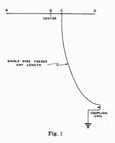
Radiation takes place essentially from the antenna wire, rather than from the feeder. At the fundamental frequency the antenna has standing waves of voltage and current, as shown in Fig. 2. The current along the feeder, under ideal conditions, would be constant—and with no standing waves of volttage or current.
