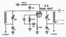
Fig. 2—Standard 6A6 oscillator-doubler circuit, the output of which is on the second harmonic of the crystal frequency.
