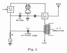
feeding a small amount of a-f voltage from the plate-modulated circuit back into the grid circuit. This resulted in better performance than the application of some plate modula-
