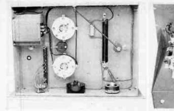
Two views of the final r-f amplifier deck, top and bottom of chasis. The grid circuit is shielded from the plate circuit by means of a large aluminum baffle.
