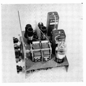
Looking into the Super-Gainer, all above-chassis components are clearly shown. The shield plate between the coils is grounded to the frame of the main tuning condenser. The 1,500-Kc. i.f. transformers are of the Meissner Mfg. Co. type, the catalog numbers being shown in the schematic wiring diagram.
