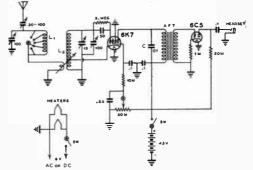
Schematic wiring diagram of highly-selective battery-operated "blooper." Values of components should not be changed. The audio transformer is a conventional 3:1 unit.
