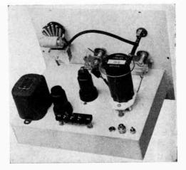
Rear view of the little "blooper," showing details of tuned antenna circuit for greater selectivity and better signal strength. Connection to antenna coil,  $L_{i}$  is by means of a pair of leads secured to the bakelite arm which rotates the coupling coil. This coil has one turn of wire, coupled loosely to coil  $L_{a}$ .
