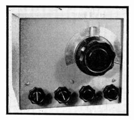
Housed in a metal cabinet only 6x6x7-in., the improved "Super Gainer" Receiver is nevertheless a full-size performer. The illustration shows the home-made vernier tuning dial, consisting of a standard dial-reduction drive coupling and 3-in. bakelite knob.
