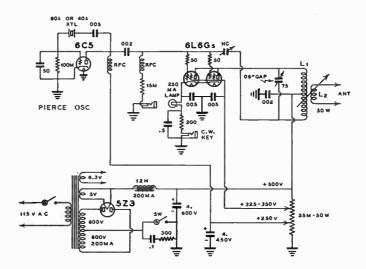
An inexpensive, compact stand-by c.w. set, complete with power supply, on a single chassis. More than 75 watts input. An ideal small transmitter for the 'phone men who wish to keep up with their code speed.
