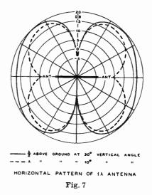
Figs. 7 and 8 show the horizontal patterns for harmonic operation. in which the wire becomes a full wave, or two full waves, at the frequency of operation. The radiation tends to become more end-fire for harmonic operation, and with less radiation at rightangles to the wire.
