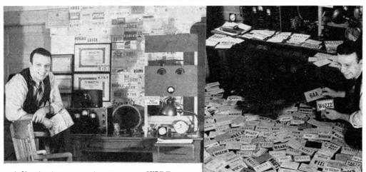
• Here's the operating spot at W7RT. Equipment includes HQ120-X receiver with home-made preselector, and an auxiliary receiver in the SW3 atop the HQ120-X. Transmitter is an 811 final with 150 watts on 40 and 20 c.w. Note two WAC certifs—from two locations, first in Seattle. and next in Goodnews Bay, Alaska, as K7RT.
