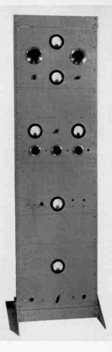
Semi-High Power, High Frequency 'Phone-C.W. Transmitter with HK-254 Gammatron Push-Pull Final Amplifier
