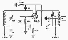
Fig. 3—Dual-triode oscillator with neutralizing circuit for the second section of the tube, thereby enabling the tube to function as a crystal oscillator and buffer or doubler.
