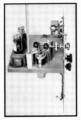
The transceiver should be thoroughly tested before it is installed in its carrying case. A temporary antenna-rod assembly is illustrated in the photograph above.
