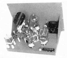
Another 75T r-f amplifier for a cathodemodulated transmitter previously built.
