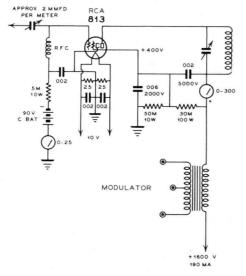
The final r-f amplifier can be biased for c.w. or 'phone operation in the manner shown above. This method is to be preferred over that shown in the tube bulletins. munication. A 150-watt modulator will then be required.
