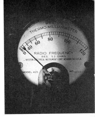
Figures don't lie. The r-f thermo-milliammeter indicates the low value of crystal r-f current in the new Wells Oscillator. Many crystal cuts were tried in this new circuit; all gave satisfactory performance—even the low-cost variety.
