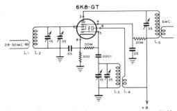
Circuit diagram of 10-meter converter. Coilwinding data is included in the general text.
