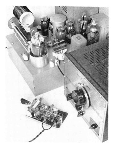
Rear view of the 813 beam tube transmitter and Meissner Signal Shifter. This medium-power compact ensemble can be quickly transported from place to place, and connected to the 110-volt a.c. mains anywhere-or to an auxiliary power plant-in order to establish emergency communication. The output of the transmitter is great enough to insure a powerful signal at the receiving point, a distinct advantage for reliable communication when and where it is needed.
