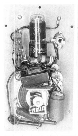
Interior view, showing midget permanent magnet loud-speaker and essential components.
