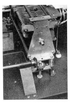
Close-up of the right-angle drive for rotating the plate tuning condenser. This arrangement makes for perfect symmetry of tuning controls on the front of the panel.
