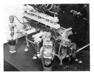
Betty's final r-f amplifier is beautifully constructed. Note particularly the rightangle gear drive for rotating the plate tuning condenser, and observe the neat arrangement of mounting the neutralizing capacitors.
