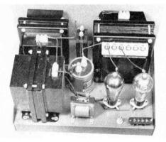
Power supply and filter for final r-f amplifier stage.
