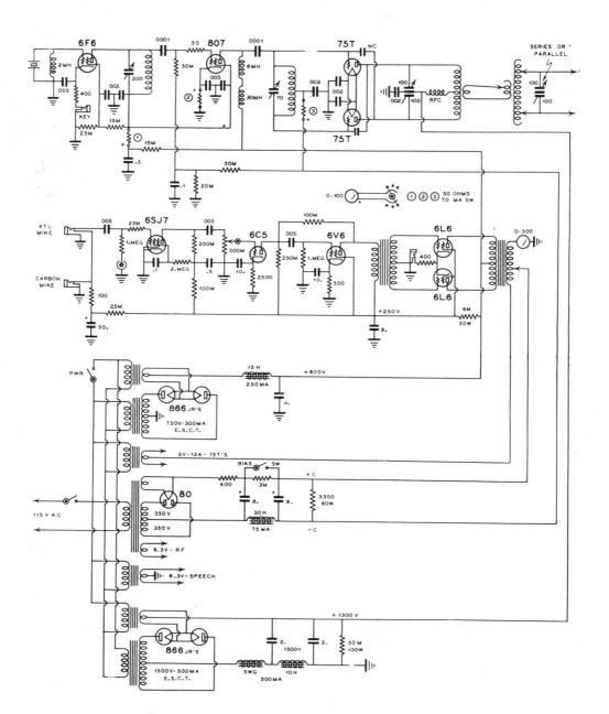
Schematic wiring diagram of 250-watt cathode-modulated 'phone and 500-watt c.w. transmitter.
