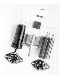
Here are the components (crystal excepted) for the new Wells Oscillator. No simpler ocsillator assembly has ever been devised.
