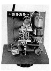
Looking into the 10-meter converter. Note mounting of tube and small components to facilitate short leads.
