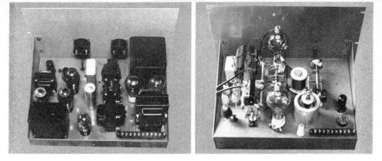
Only two chasses are required for the exciter, final r-f amplifier, speech channel and its power supply. The illustrations show the principal components for a compact mediumpower cathode-modulated transmitter, described in the text.
