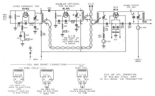
Complete schematic wiring diagram of the 813 beam-tube transmitter and supplementary sketches showing coil connections for ECO or crystal operation.
