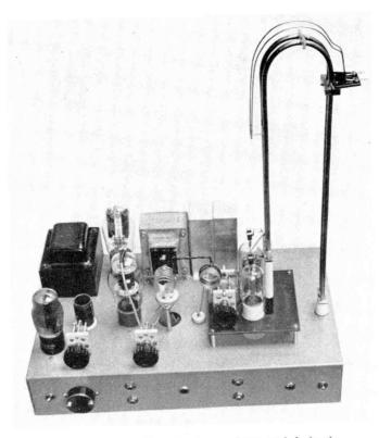
The complete  $2^{1/2}$ -meter transmitter and hair-pin rod assembly.
