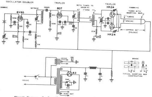
Circuit diagram of r-f portion of  $2^{1/2}$ -meter crystal-controlled transmitter.
