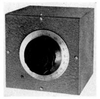
Front view of the 10meter converter. A vernier tuning dial is a convenience for covering the congested band.
