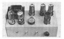
Top view of miniature c.w. transmitter, showing small BC transformer, tubes, and final r-f plate coil.
