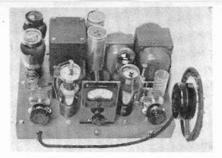
Low power 10- and 20-meter r-f unit and modulator for operation from VFO or crystal oscillator. All of the components are mounted on a chassis only 12-in. x 10-in. If you want a small 'phone transmitter, one which has been correctly engineered, here it is.
