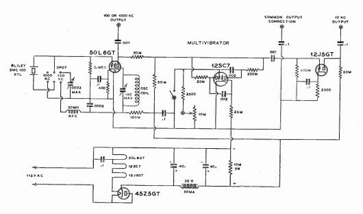
Wiring diagram of the Frequency Standard. Values of components are critical and should be adhered to rigidly by the constructor. These values were determined after painstaking research in the laboratory of the author.
