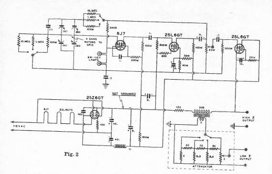
Both R/C oscillators include a 25Z6GT voltage-doubling rectifier in order to obtain a +B potential of from 175 to 300 volts from the 115-volt a.c. line.
