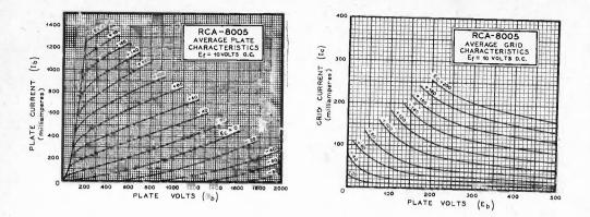
As R.F. Power Amplifier—Class B Telephony Carrier conditions per tube for use with a maximum modulation factor of 1.0
