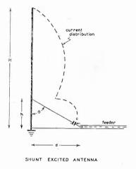
matched properly by varying the connection point on the inclined conductor, i.e., the distance h. The capacity C can then be varied until the transmitter load becomes normal, and then the standing waves are minimized or eliminated from the transmission line.
