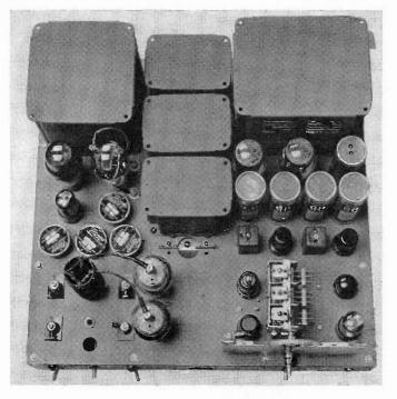
Expert workmanship is evidenced by this transmitter-receiver for defense service. The final r-f amplifier has a pair of Hytron HY-59 tubes, modulated by a Hytron HY-31Z. The transmitter portion has four crystals, each on a spot frequency, yet the amateur may contend himself with but a single crystal.
