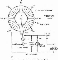
Resistor-box connections for indicating device.
