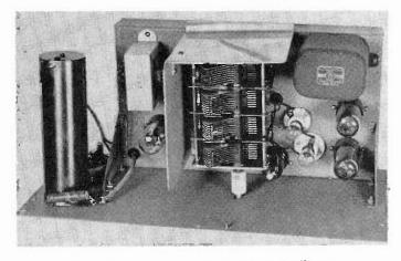
Interior view of capacitor-type R-C Oscillator.
