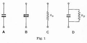
Consider a perfect condenser as shown in Fig. 1a. This would consist of two metal plates with no insulation but air between them. In such a case the current in the condenser would be exactly 90 degrees out of
