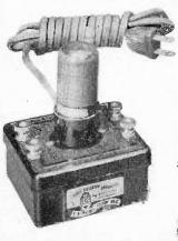
Oscillatone, ex-cept smaller housing because no speaker. Elec-tronically keyed, which means limitless speed and clean keying. Uses 110 to 120 volts, either AC or DC. Connect jumper wire across two rear terminals for speaker speaker volume. Terminals: 2 right for key left for headkey: 2 phones.
