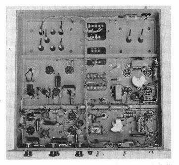
The professional version of the transmitter-receiver is built upon a heavy cast aluminum chassis, divided into six compartments on the under side. A more simple chassis construction for amateur service could be a conventional steel deck with suitable reinforcing frames below.
